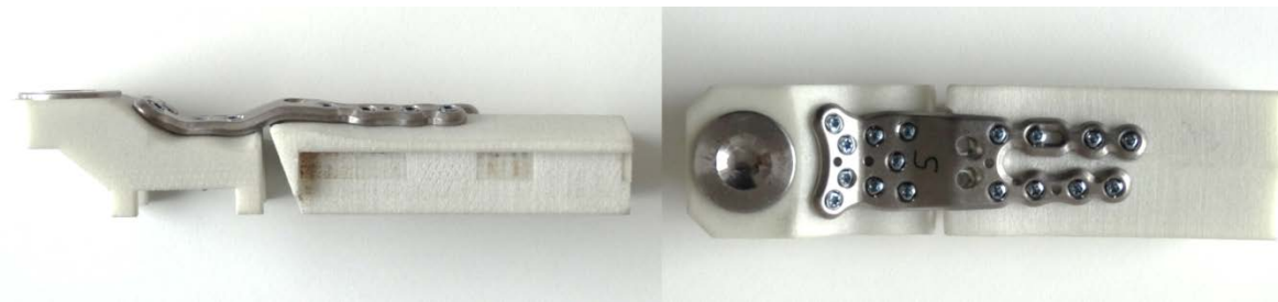
Fatigue test: Comparison between commercially machined plates and SLM plates.
