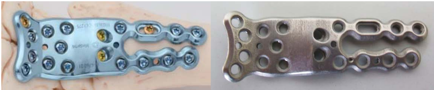
Left: Medartis® wrist fusion plate spanning the radio-carpal and mid-carpal joint. Right: SLM replica.
